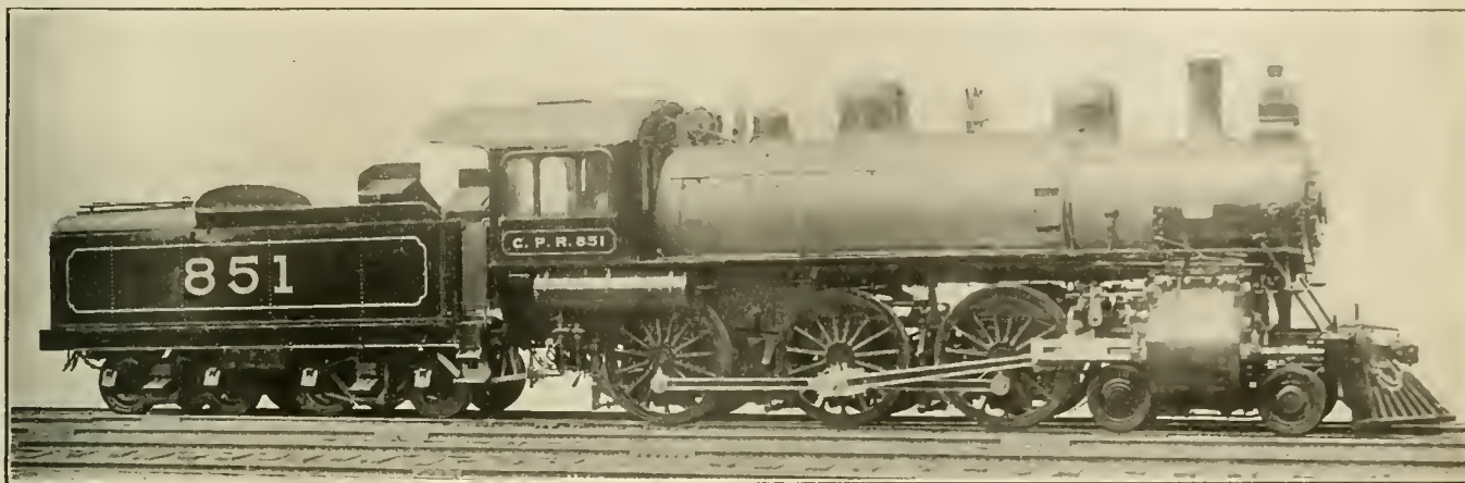
TEN-WHEEL COMPOUND LOCOMOTIVE—CANADIAN PACIFIC RAILWAY
